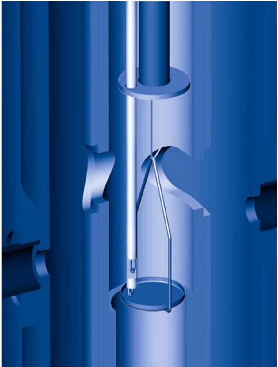
The same thermocouple used for accurate measurement of the sample temperature is also used for controlling the furnace. The benefit of this unique capability is a highly responsive furnace. In particular, this design provides superior isothermal temperature control. A second thermocouple in the same ceramic sleeve is a backup thermocouple for safety purposes.
